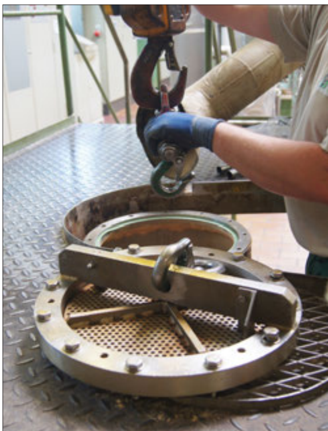
Left: Loading Extractor vessel CO2, Right: Ginger CO2 extract homogenization © Madeleine Kerkhof, Kicozo
